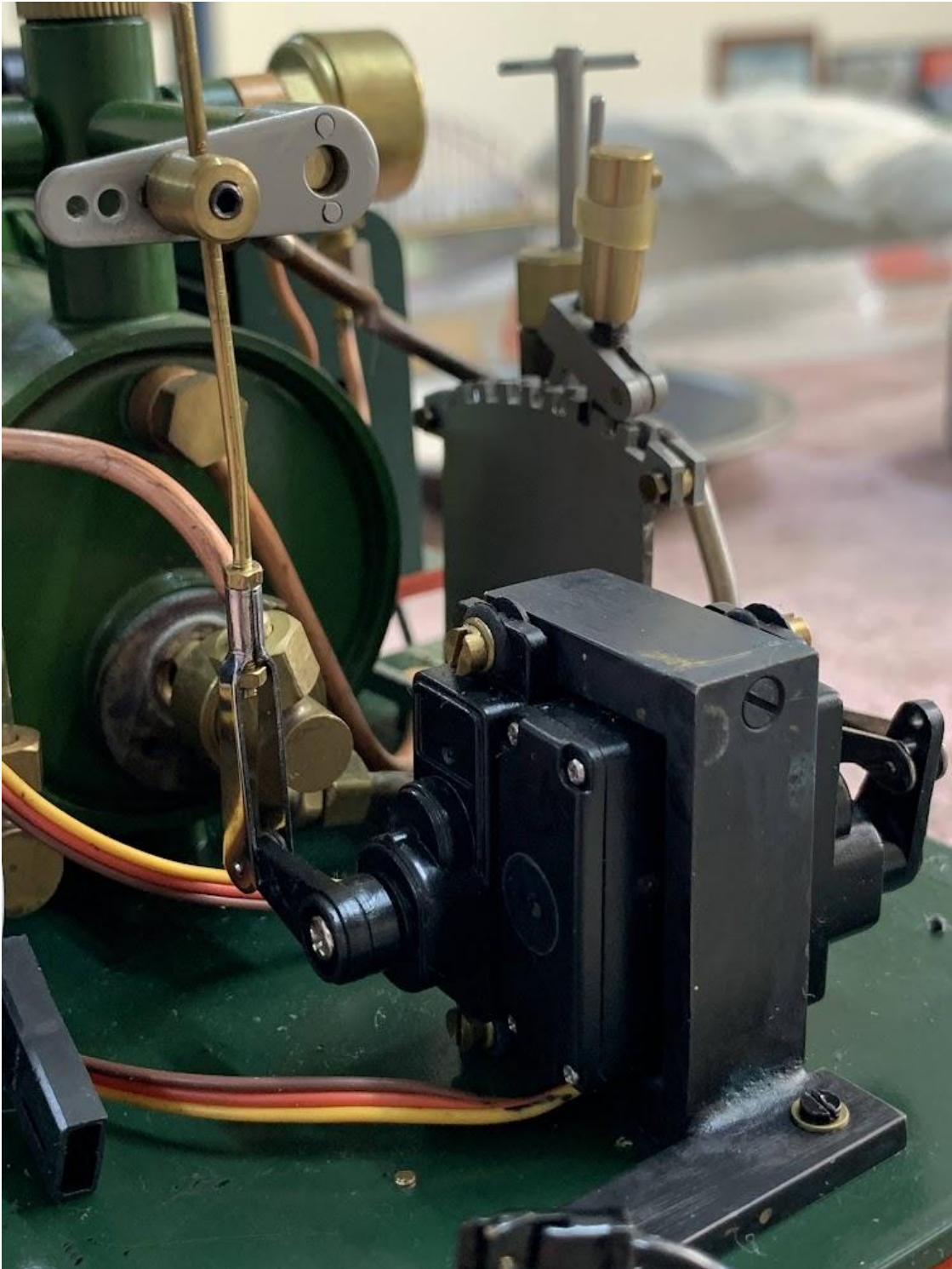
Servo connection to the steam regulator
