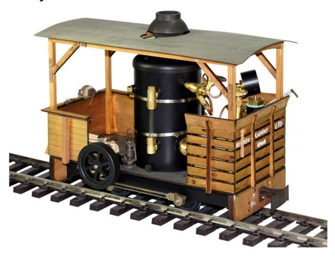
Henry is a live steam freelance locomotive based on American logging tradition. Supplied as a kit, the major assemblies (boiler, engine unit, gas tank) are prefinished leaving you to assemble the chassis, wooden body, plumbing etc. Controls include steam regulator, reverser, water level gauge, pressure gauge. Powered by a single, double acting oscillating cylinder, flywheel and a geared drive to the wheels. Wheels are insulated and are gauge adjustable..
