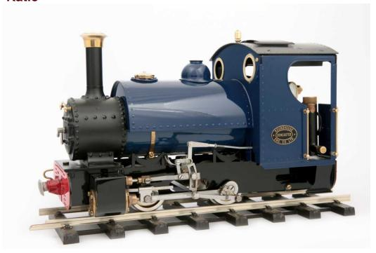
Katie is of typical narrow-gauge saddle tank locomotive design. Though not a model of any particular engine, she draws inspiration and features from a number of famous builders like Hunslet, Bagnall and Pecket etc.
