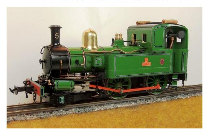
Arriving as a joint delivery with No. 4 Loch in 1874 in readiness for the opening of the Port Erin line, the locomotive is named from the Latin word meaning Isle of Man. Together with sister No. 4 she carried unusual nameplates to compensate for the injector overflow pipe which bisected it, thus the name appears 'MO NA' with a gap to allow for the copper pipe; modifications to the layout leaving this feature redundant and giving it an unusual appearance.
