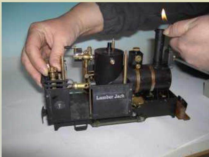
Prior to ignition open the gas cock briefly and listen to determine whether the burner is blowing cleanly. If it is sputtering then discharge a little gas via the fill pin until a clean jet is audible.
