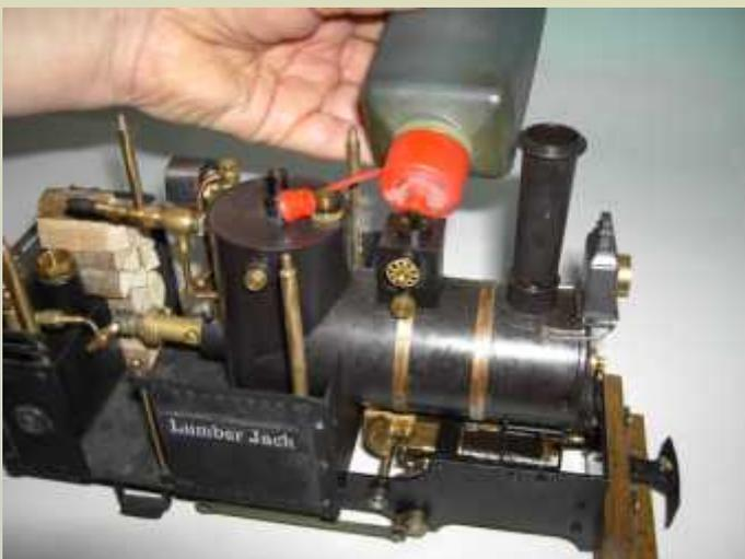
Unscrew the lid of the oiler and fill with steam oil to the level of the adjustment spindle. Do not use any other oil. Steam oil is not washed off by the steam. It contains tallow which resists being washed away and in addition it has a supplemental sealing effect. A different type of oil could lead to premature wear, or in the worst case, it could cause the pistons to jam. Now screw on the oiler lid again.
