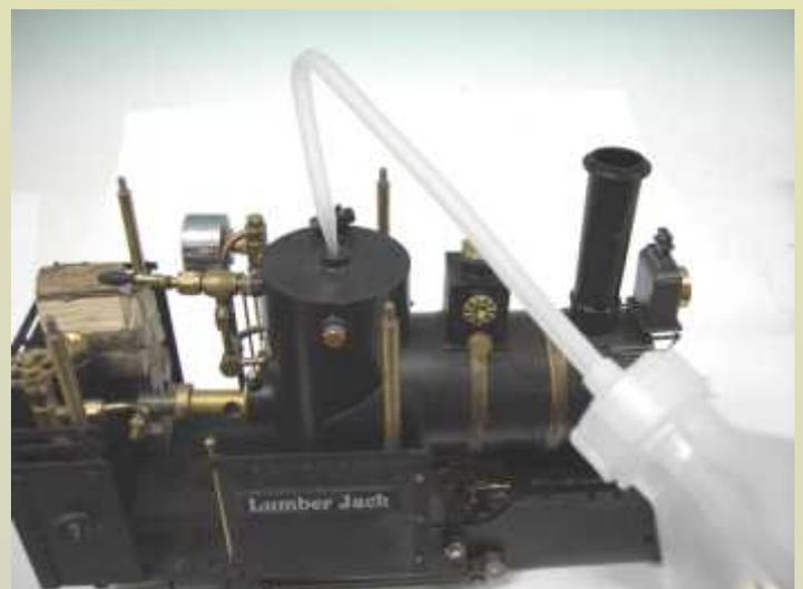
Unscrew the pressure control valve. Use the water bottle to add water to approximately 2/3 of the height of the glass tube. Use distilled water, to which 3-5% tap water has been added. This minimizes the aggressive characteristics of distilled water and allows residual water to be able to be left in the boiler without draining for storage or inactive periods without resulting in the dreaded pitting.
