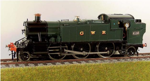
Ideally suited for suburban and branch line work, The 61XX variant was introduced in 1931 and was little different from its predecessors apart from boasting a boiler pressure increased to 225psi. A number of 51XX and 41XX examples have been preserved but only 6106 was saved from the last batch and this can be found at Didcot, home of the Great Western Society.
